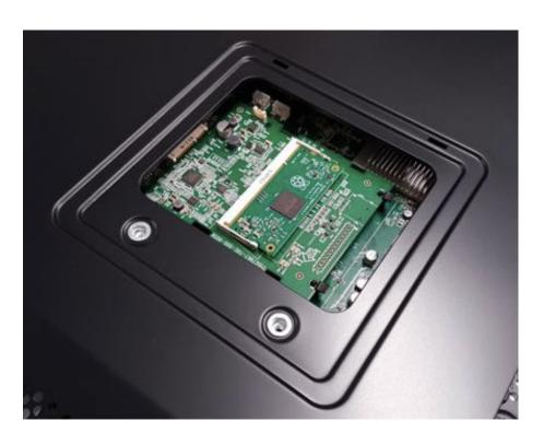
Many people want to embed Raspberry Pi into their own product. To help them, we produced the "Compute Module". This is a Raspberry Pi on a small SO-DIMM PCB, which fits into a socket on the main product PCB.
