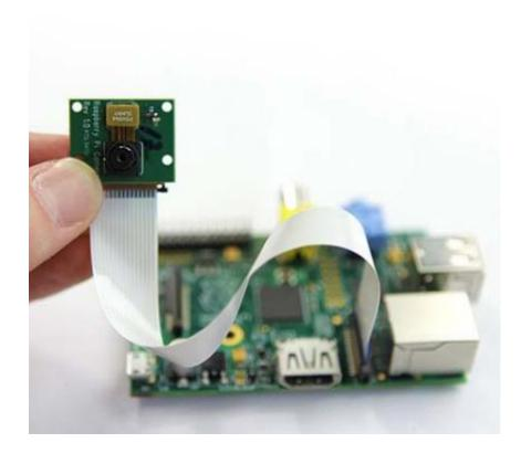
The Broadcom BCM2835 chip in the Raspberry Pi has a very powerful image processor, which has been used in many high-end Nokia camera phones. Two weeks ago, we launched a \$25 accessory which adds a fixed-focus camera module. This is able to capture 5megapixel JPEG images, or record HD video at 30 frames per second. We are excited to see what people do with this capability over the next year
